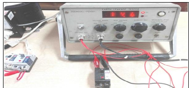
Fig. 2. Operating time measurement of ELCB
