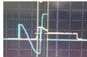
Fig. 9. Measured waveform of entire operation time of circuit-breaker
